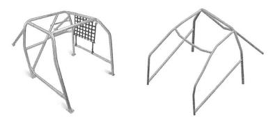
\*Cage will need to be at a minimum 1 ½ .095 tubing with 1/8" thick plate welded or bolted to the body. \*Correct mounting of racing seats is attaching them to the factory seat mounts brackets or to the roll cage. Seats & belts must be mounted to the cage for Limited-Pro, Pro-Stock, & Outlaw.
